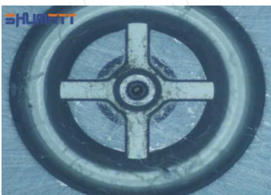
Obvious Wear marks on edge
